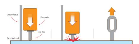
Aluminum Key is placed in the electrode fixture. Bring the Key in contact with the dent. Ground Stud should be in contact with the base material as well.
